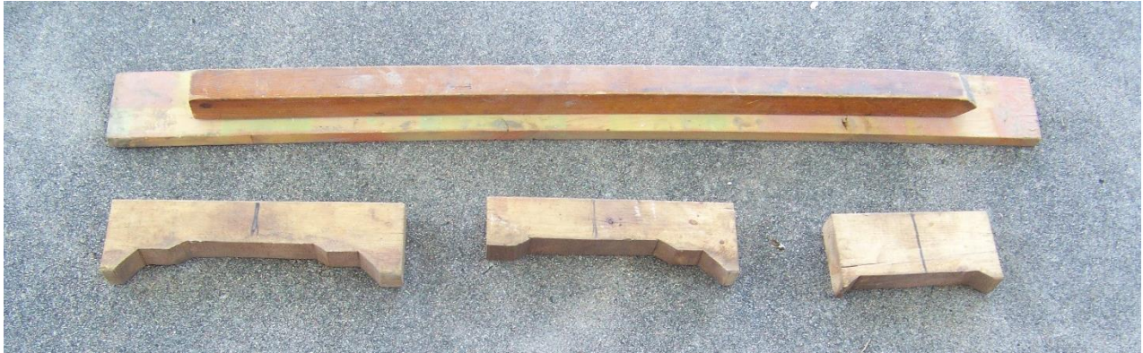
Templates and float used for Roadbed
